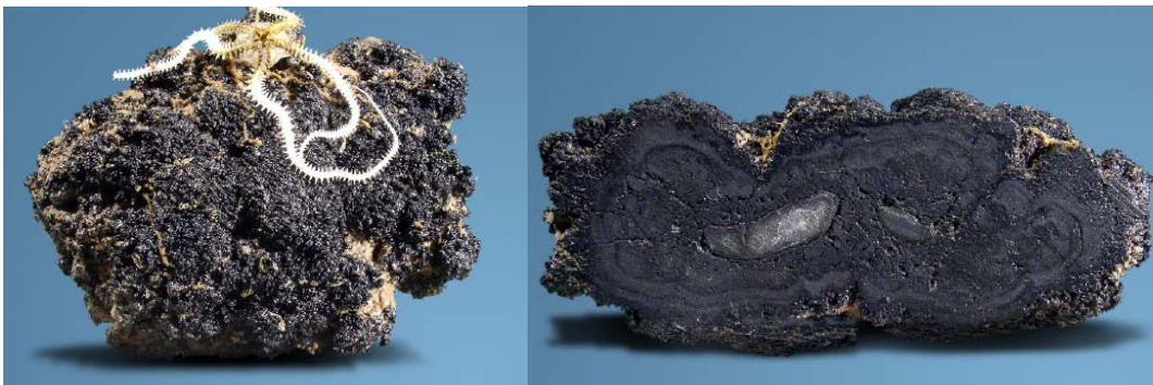
Figure 1. Mn-rich polymetallic nodules (about 30 cm each) from the exploration area of the Interoceanmetal Joint Organization in the Clarion-Clipperton Zone (received from R. Kotlinski)
